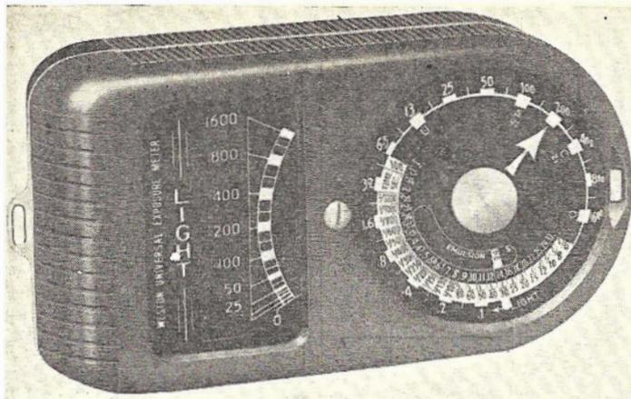
Accurate measurements in weak light, automatically changing "high light" and "low light" scales, increased number of exposure values, and sharply directional viewing angle are some of the features of a new photoelectric exposure meter, intended for general photographic purposes. The molded case and open face dials make the instrument easy to use.
