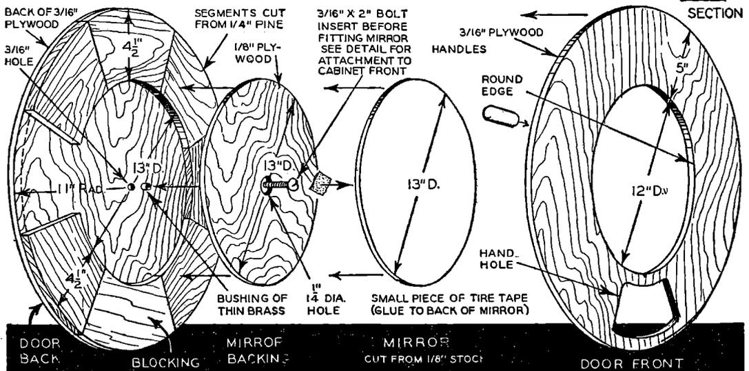
AND REVOLVING DOOR - GLUE DOOR PARTS TOGETHER IN ORDER SHOWN AND CLAMP -
