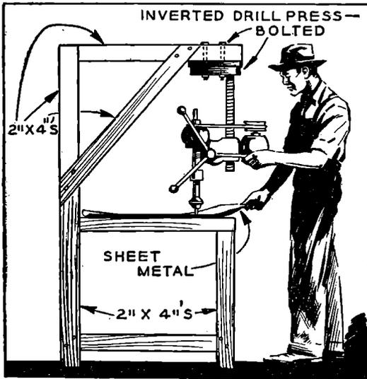
**A** ROADSIDE sign specialist rigged up a medium size bench type drill press in an upside down position to permit the quick boring of holes to the center of 5 foot squares and circles. The installation is unusually simple and effective, as shown above.
