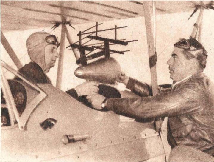
Above: Pursuit plane uses beam to spot oncoming enemy bombers in darkness. Left: Inventor takes up apparatus to test its efficiency in flight. Below: In demonstration, sensytrol beam on ground locates and records on voltmeter presence of plane in air above airport.
