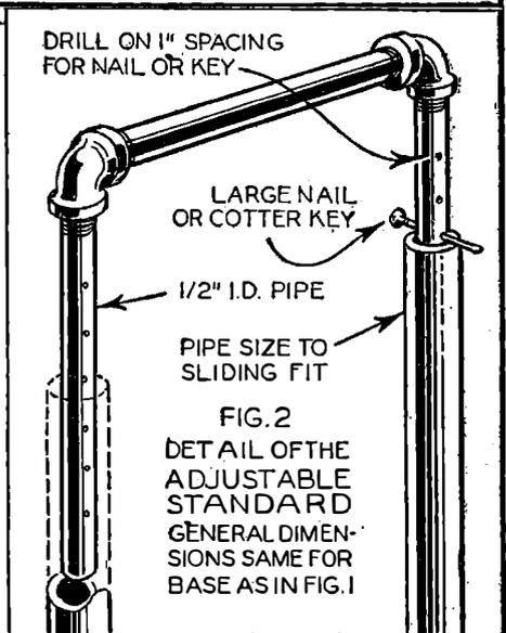
FIG. 2 DETAIL OF THE ADJUSTABLE STANDARD GENERAL DIMENSIONS SAME FOR BASE AS IN FIG. 1
