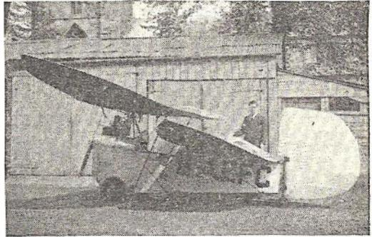
J. G. Crampton is the builder of this Flying Flea plane. It is powered with a four-cylinder, water cooled engine and the main plane has a span of 21 feet. In England, where Crampton lives, home-made airplanes are permitted.
