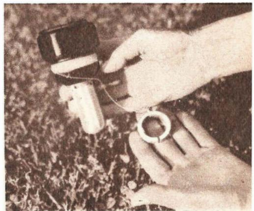
A midget buoy to mark the spot where fish bite best. As lead ring sinks, the line unreels from head of buoy until bottom is struck, then engages tiny hook at one side to eliminate more unwinding. The metal tube, perforated with holes, fills with water, causing buoy to bob upright.
