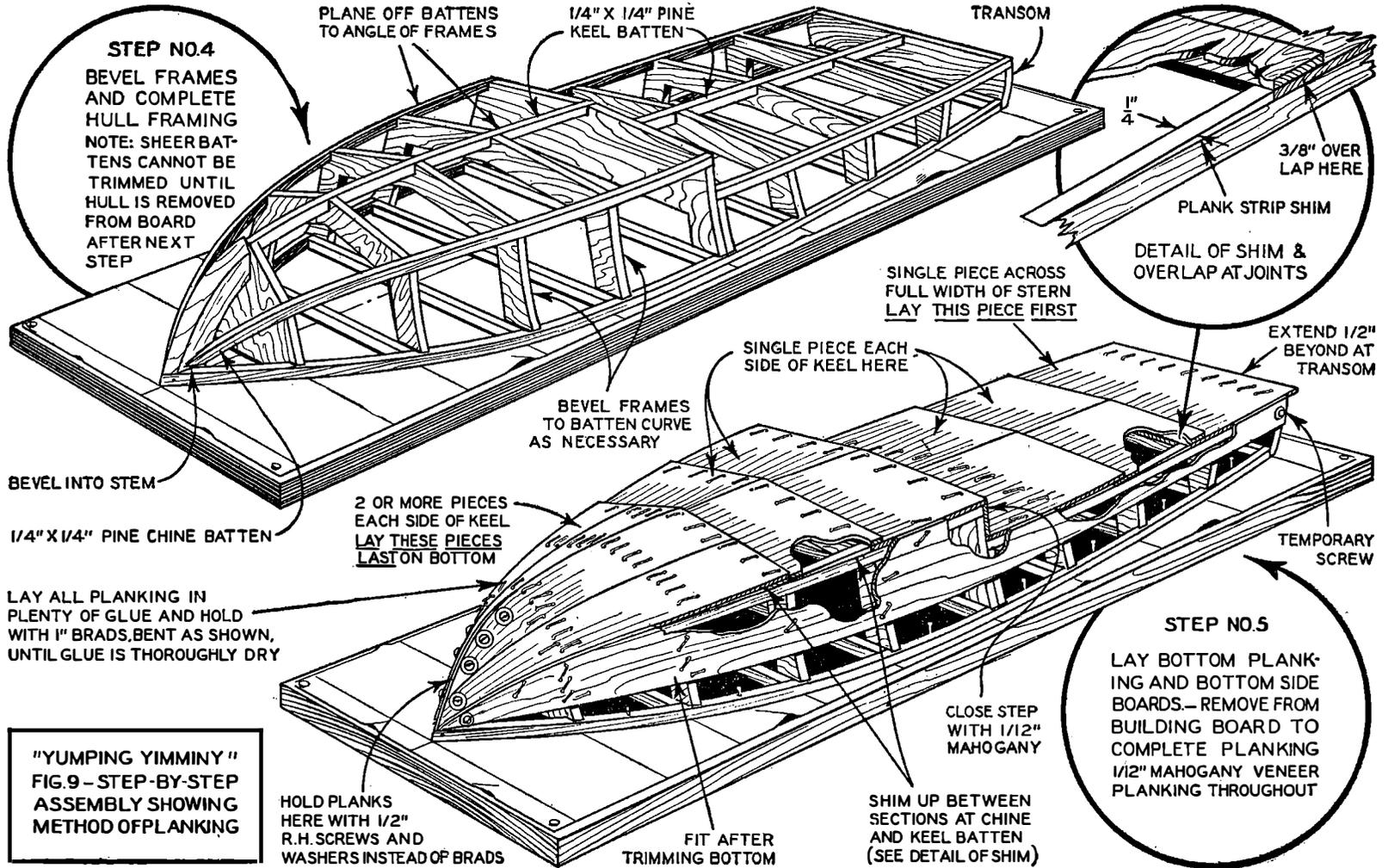
Top: Framing complete with chines and keel in place. Frames are beveled and bottom is ready to be planked. Lower drawing clearly shows method of planking. Mahogany veneer is laid in glue, held down with brads until dry except at stem, where twist of planks makes it necessary to use screws.
