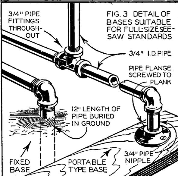
FIG. 3 DETAIL OF BASES SUITABLE FOR FULL-SIZE SEE-SAW STANDARDS
