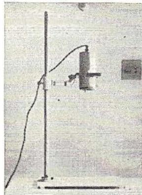
This photo of an enlarger built from MI plans by Leonard Prehn was taken with a miniature camera and "blown up" by the home-made enlarger.
