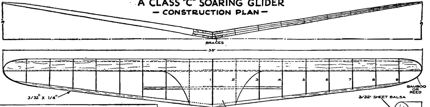
WING RIBS. CUT 2 OF EACH FROM 1/16" SHEET Balsa.
