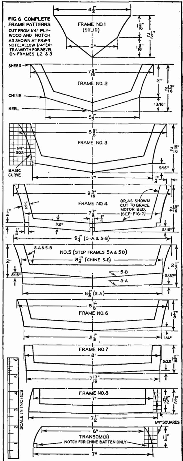
All frame patterns are given at right. They should be copied full size on paper, pasted to plywood and cut out to line. Beveling takes place later.
