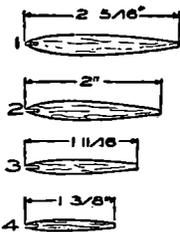
TAIL RIBS. CUT 2 OF EACH FROM 1/16" SHEET. NO. 1 IS OF 1/8" SHEET.
