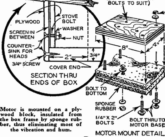
Motor is mounted on a plywood block, insulated from the box frame by sponge rubber, thus eliminating most of the vibration and hum.
