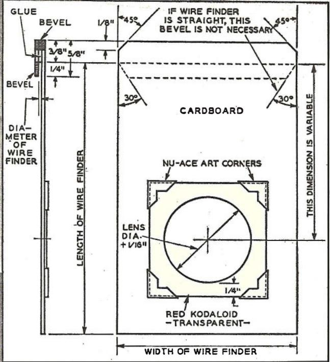
**W**HEN film pack cameras are used as horizontal enlargers a filter holder to hold a red filter over the camera lens while enlarging is essential. This allows the photographer to place the sensitized enlarging paper in the printing frame or paper holder without danger of fogging, and also for final adjustment.
