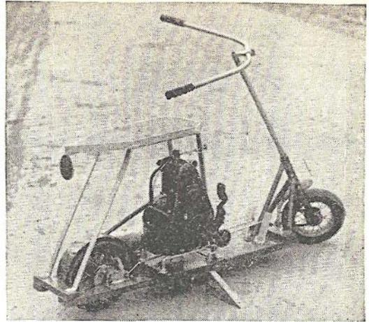
A motor scooter powered with a washing machine engine is the work of Leo VanBenthusen. Built at a cost of \$18, it will do 60 miles on a gallon of gasoline and has a top speed of 18 miles per hour.
