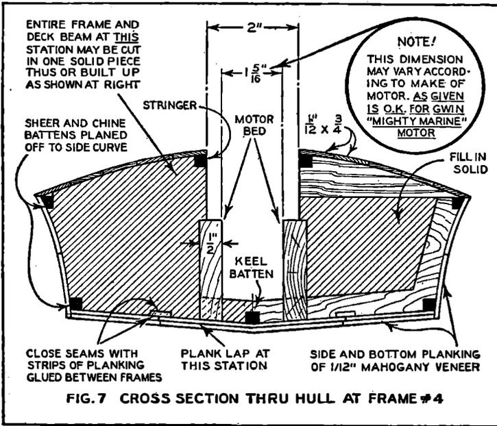
FIG. 7 CROSS SECTION THRU HULL AT FRAME #4
