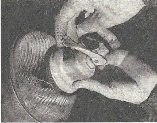
A suction tool strong enough to pick up 40 pounds dead weight is handy for the auto mechanic. It is designed especially for removing glass parts or hub caps and for pulling out soft dents in car bodies.
