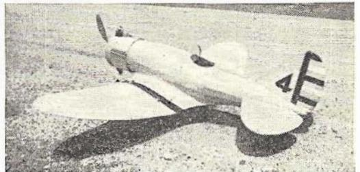
This low wing gasoline model airplane is the work of J. A. Williams. It is powered by a 1/2 horse power engine and has a wing span of 42 inches.
