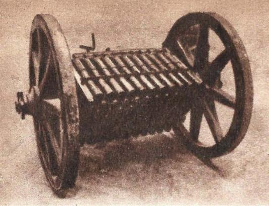
Pre-dating the anti-aircraft gun shown at the right was this multiple-barreled gun designed by da Vinci to fire successive volleys.
