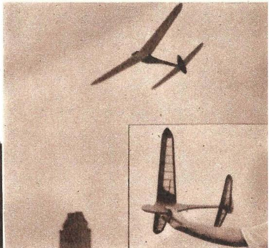
**Contest Gliders.** Original designs for the three popular gliding model classes. At left, Class A and B solid balsa gliders. Above, Class C hollow-wing sailplane. Page 100.
