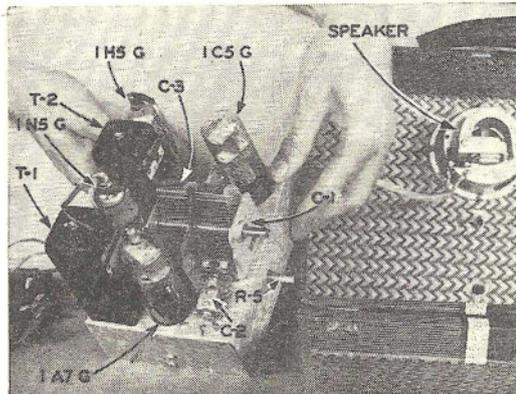
Distribution of the parts on the top of the chassis of the "Picnic Portable." In mounting the speaker in the face of the overnight bag, make sure it clears the movable plates of the tuning condenser C1-C3.
