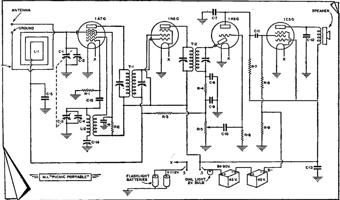
In this schematic diagram of the "Picnic Portable," the two small switches marked "S" are actually one double-pole, single-throw unit mounted on the back of the volume control R5.
