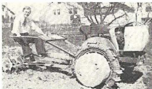
Roger Fredsall constructed this chain drive tractor from an old motorcycle engine and parts of old cars. It cost only \$10.
