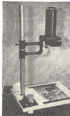
This enlarger is the work of Fred Van Egy of Oakland, Calif. It will cover up to a 2 x 2 inch negative. Fred's own picture is being enlarged in the photograph.
