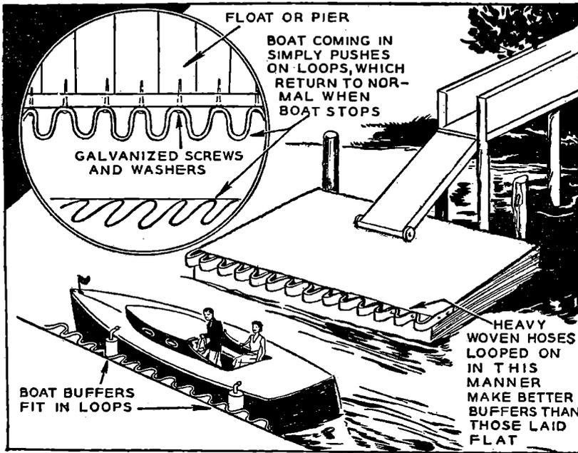
**A**N EXTREMELY effective pier or float buffer can be made with a length of old firehose. Nail or screw it to the edge of the dock in loops, as shown at left. The resilient hose will give as a boat comes alongside, effectively preventing scuffing or scraping of painted or polished sides. The loops also act to engage the round buffers generally hung over the boat's side when approaching landing, thus steadying it considerably when tied to float.—Hi Sibley.
