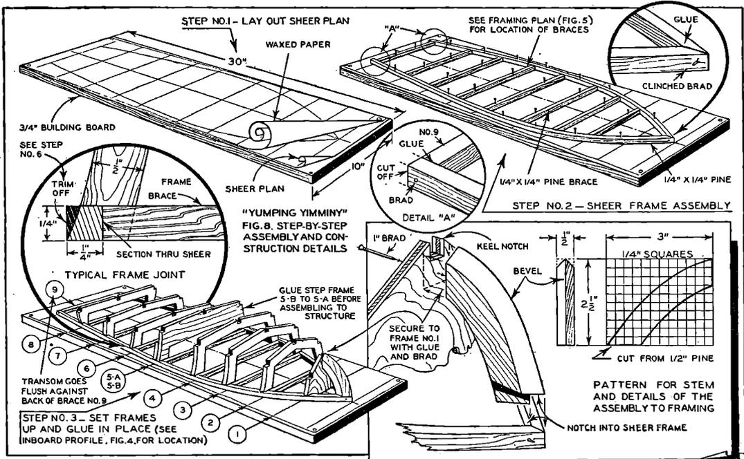
Step by step assembly drawings start above. After sheer frame has been glued together set up the frames at their various stations, drawn on your plan beneath the waxed paper. Glue in place, then cut stem and mount between sheer frame and frame No. 1 (forward bulkhead).
